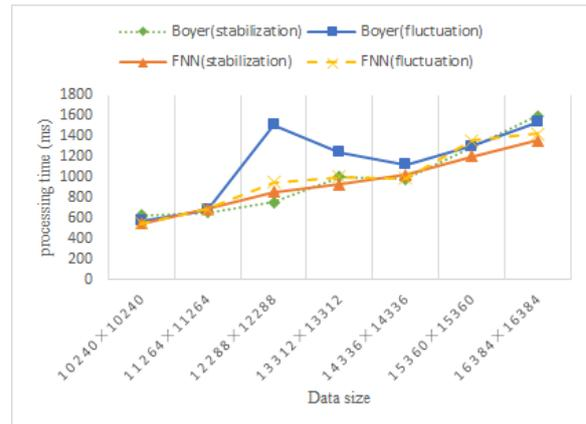
Fig. 9 The comparison of processing times between FNN based DLB model and the Boyer’s model
