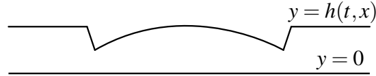
Figure 3: Geometry of the simple ‘flat’ model. Instead of two curved surfaces, the model has one flat surface, y = 0 , and one curved surface, y = h(t, x) (not to scale).
