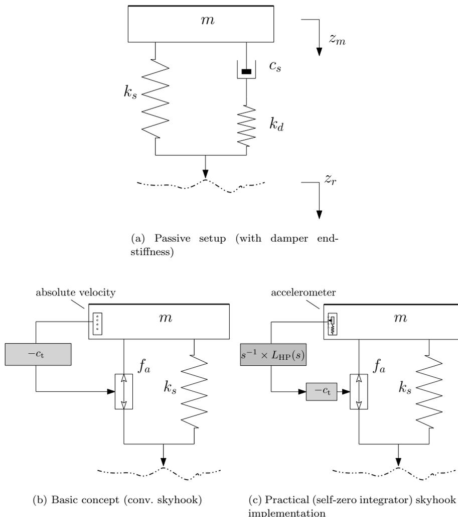
Figure 1. Passive and skyhook damping control schemes
