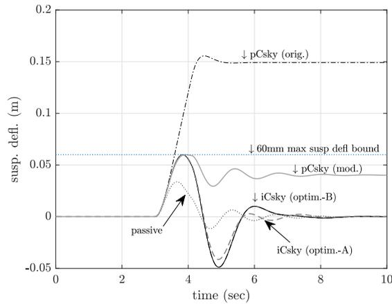
Figure 4. Suspension deflection conventional skyhook damping schemes (deterministic)
