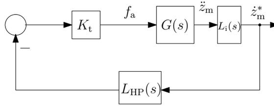
Figure 2. Feedback setup for implemented skyhook scheme
