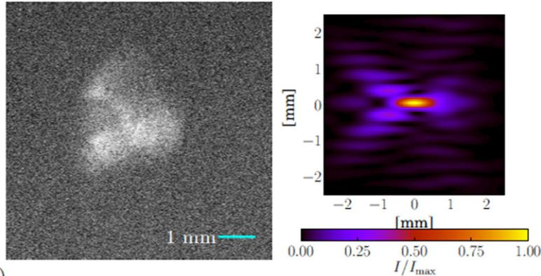
**Fig. 4** A measured profile of the EUV laser (left) and a simulated profile (right) transmitted through a parylene target of thickness 1028 nm. The transmitted EUV laser light is collected with a multi-layer mirror which is identically positioned as a multilayer mirror used to focus the EUV laser onto the target. Transmission of EUV light only occurs when the target has been ablated through the total target thickness.
