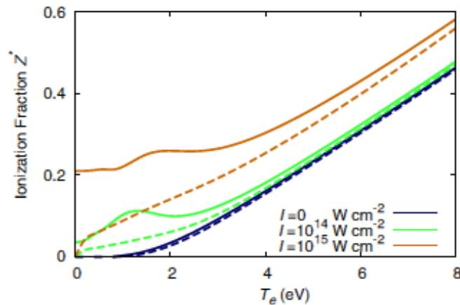
**Fig. 5** The steady state ionization  $Z^*$  of a carbon plasma at solid density irradiated by EUV photons of energy 50 eV at the indicated irradiance as a function of electron temperature. The free electron distribution is assumed to be Fermi-Dirac (solid curves) or Maxwellian (broken curves).
