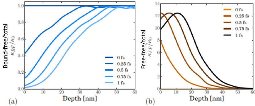
**Fig. 2** The contribution to the absorption coefficient due to (a) photo-ionization and (b) inverse bremsstrahlung for solid density carbon irradiated by photons at irradiance  $10^{14}$   $\text{Wcm}^{-2}$  and photon energy 26.4 eV at times indicated. The absorption coefficients are normalised to the photo-ionization coefficient for neutral carbon.
