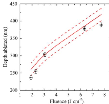
**Fig. 3** Comparison between experimental ablated depth measurements (squares) and simulations (solid line) as a function of EUV laser fluence on target. The dashed line indicate the resolution of the Eulerian mesh used in the simulations. Each data point represents the ablation depth for a single shot at the indicated fluence which was determined from the area of the ablated surface.
