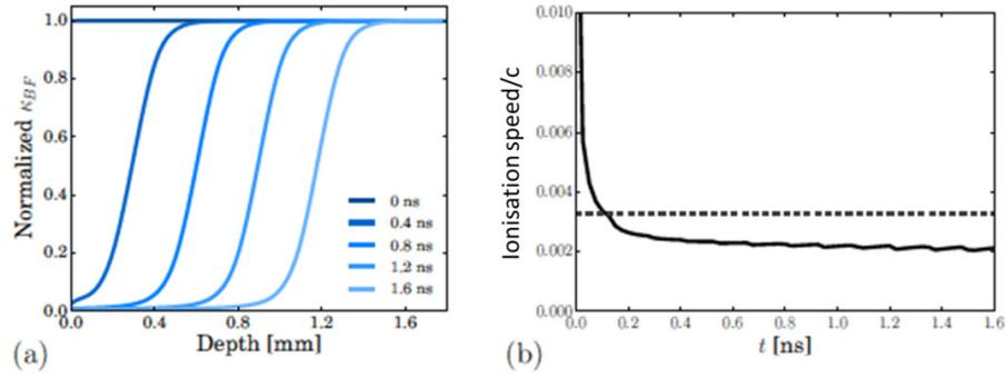
**Fig. 1** (a) The normalised photoionization absorption coefficient of helium at atmospheric pressure during irradiation by a laser pulse with a flat temporal profile and photon energy 26.4 eV at irradiance of  $10^{10}$  Wcm<sup>-2</sup>. (b) Simulated speed of propagation of the ionisation wave  $dx/dt$  (solid), determined as the point where the normalised absorption coefficient takes a value of 0.5, compared to the value following equation (2) assuming zero particle temperature (dashed).
