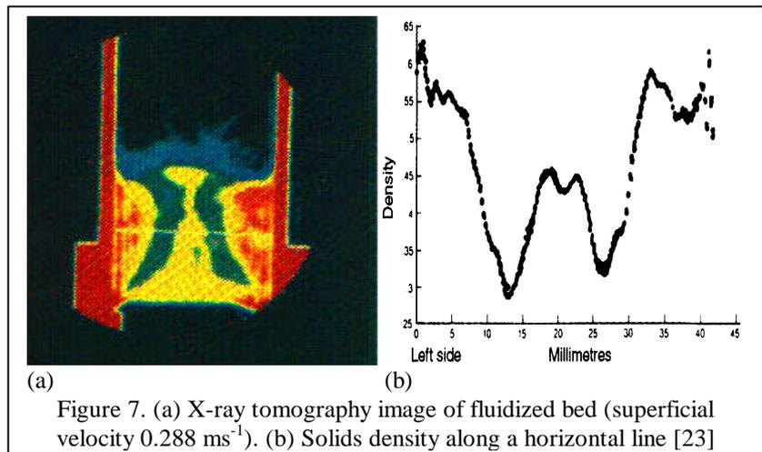
Figure 7. (a) X-ray tomography image of fluidized bed (superficial velocity  $0.288 \text{ ms}^{-1}$ ). (b) Solids density along a horizontal line [23]
