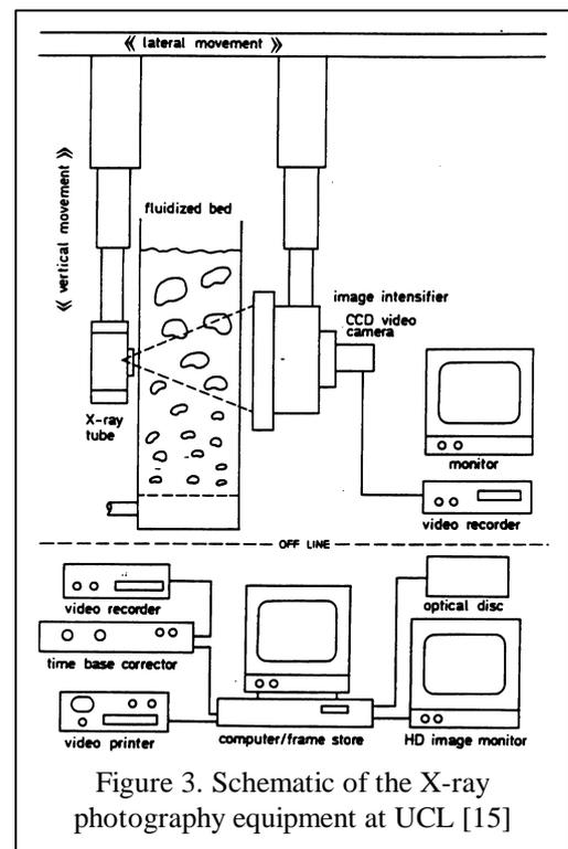
Figure 3. Schematic of the X-ray photography equipment at UCL [15]
