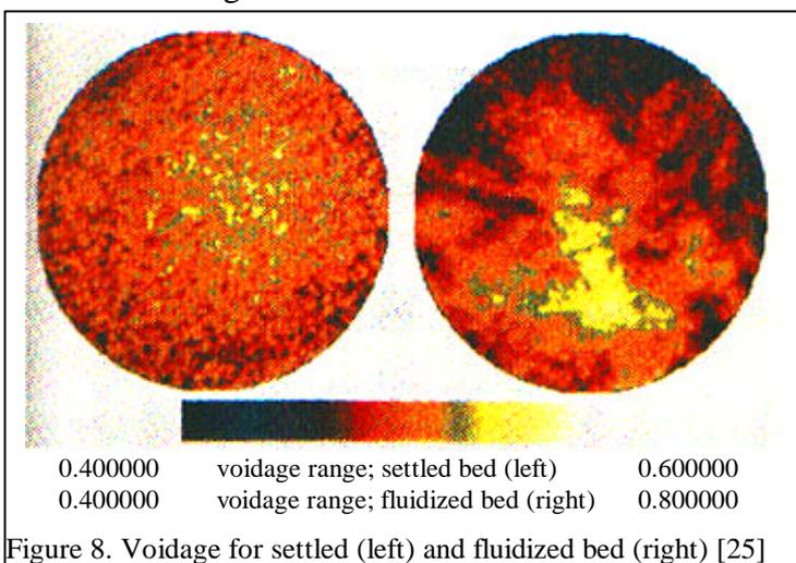
Figure 8. Voidage for settled (left) and fluidized bed (right) [25]
