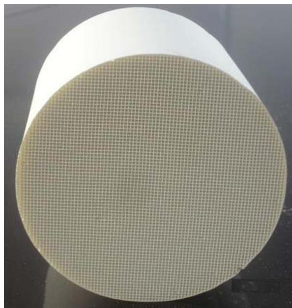
Fig. 3 The ceramic regenerator
