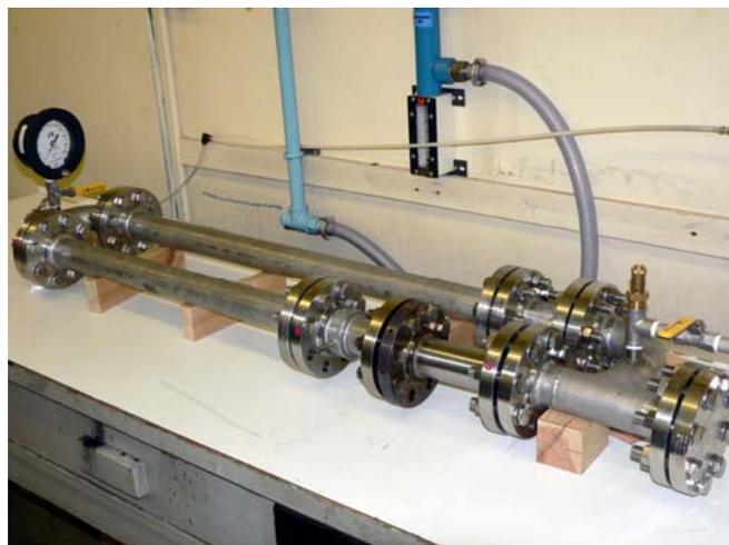
Fig. 2 Looped tube travelling-wave thermoacoustic engine
