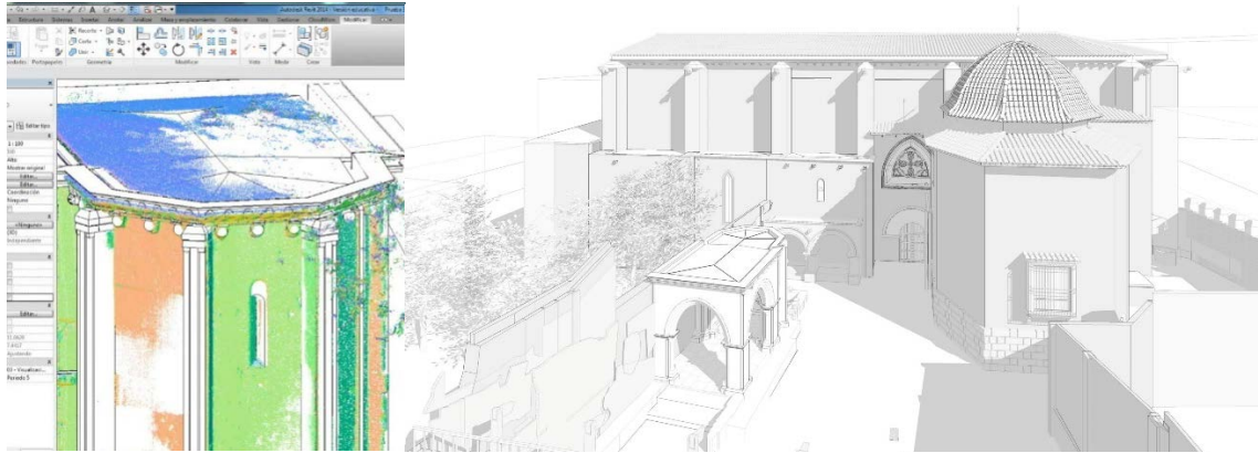
Figure 9. Modelling process based on the point cloud previously created.
