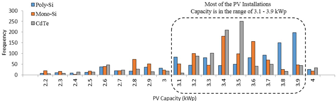
Fig. 4. Distribution of the PV installations capacity.
