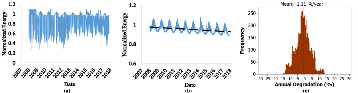
Fig. 1. Example of the YOY degradation process. (a) Data filtering, (b) Aggregation process, (c) Output degradation analysis.
