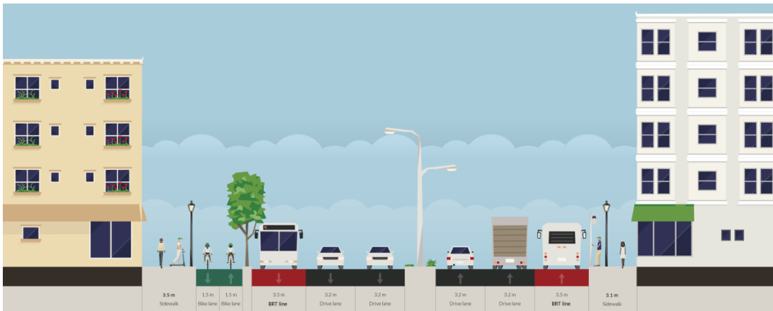
Figure 6: Proposed cross section for an arterial with public transport priority-MP (Example Width: 32m) | Image source; authors' own elaboration on Streetmix online software tool)
