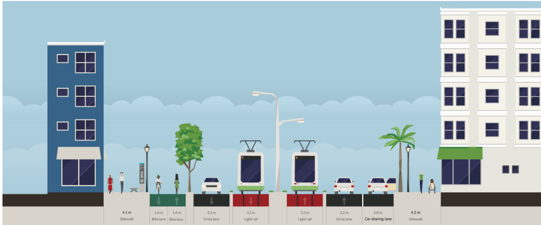
Figure 7: Proposed cross section for an arterial with sustainable modes priority-MS (Example Width: 30m) | Image source; authors' own elaboration on Streetmix online software tool)
