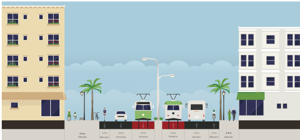
Figure 8: Proposed cross section for a boulevard with public transport priority-CM (Example Width: 25m) | Image source; authors' own elaboration on Streetmix online software tool)
