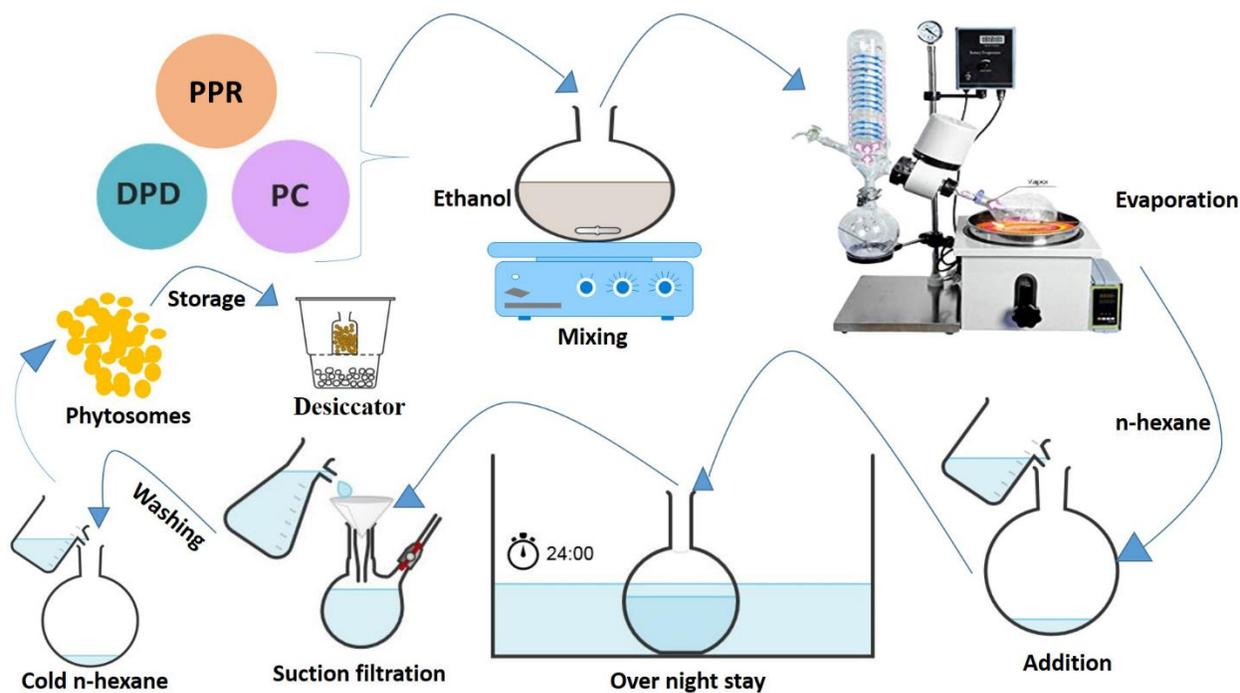
**Figure 1.** Schematic diagram of manufacturing process of phytosomes.
