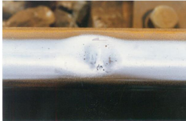
Figure 1: Typical squat defect [3]
