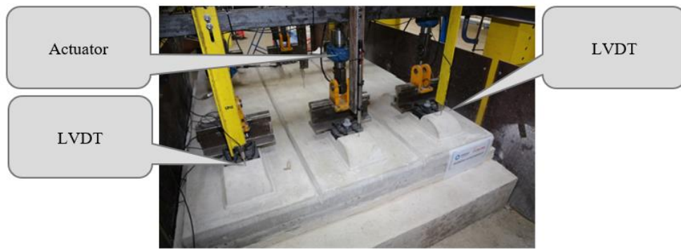
Figure 2 – GRAFT II test facility - Actuators and LVDTs
