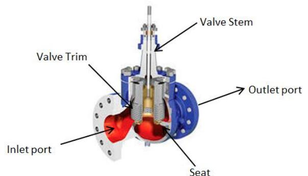
Figure 1: Components of a control valve with trim [1]
