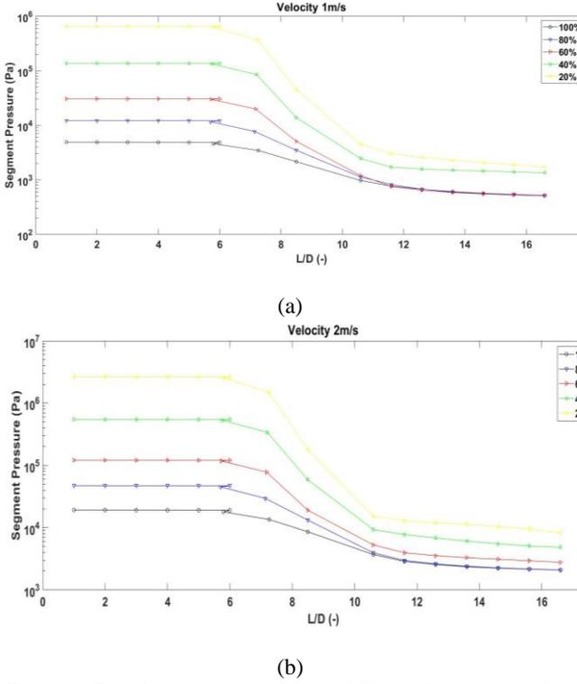
Figure 6: Local segment pressure at different locations within the valve at 20%,40%, 60% ,80% and 100% VOP with a) 1 m/s inlet velocity (b) 2 m/s inlet velocity
