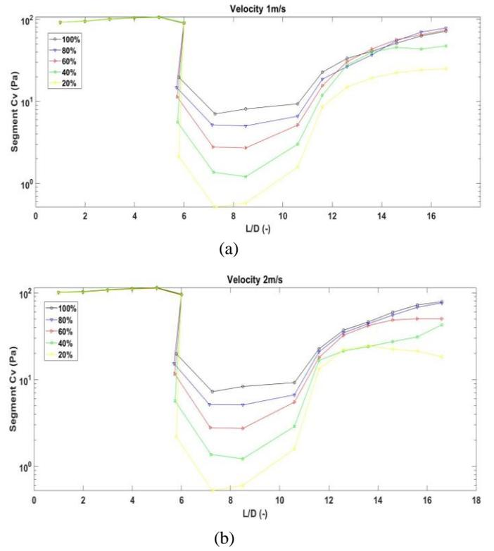
Figure 7: (a) Local flow coefficient  $C_v$  at 1 m/s inlet velocity (b) Local flow coefficient  $C_v$  at 2 m/s inlet velocity
