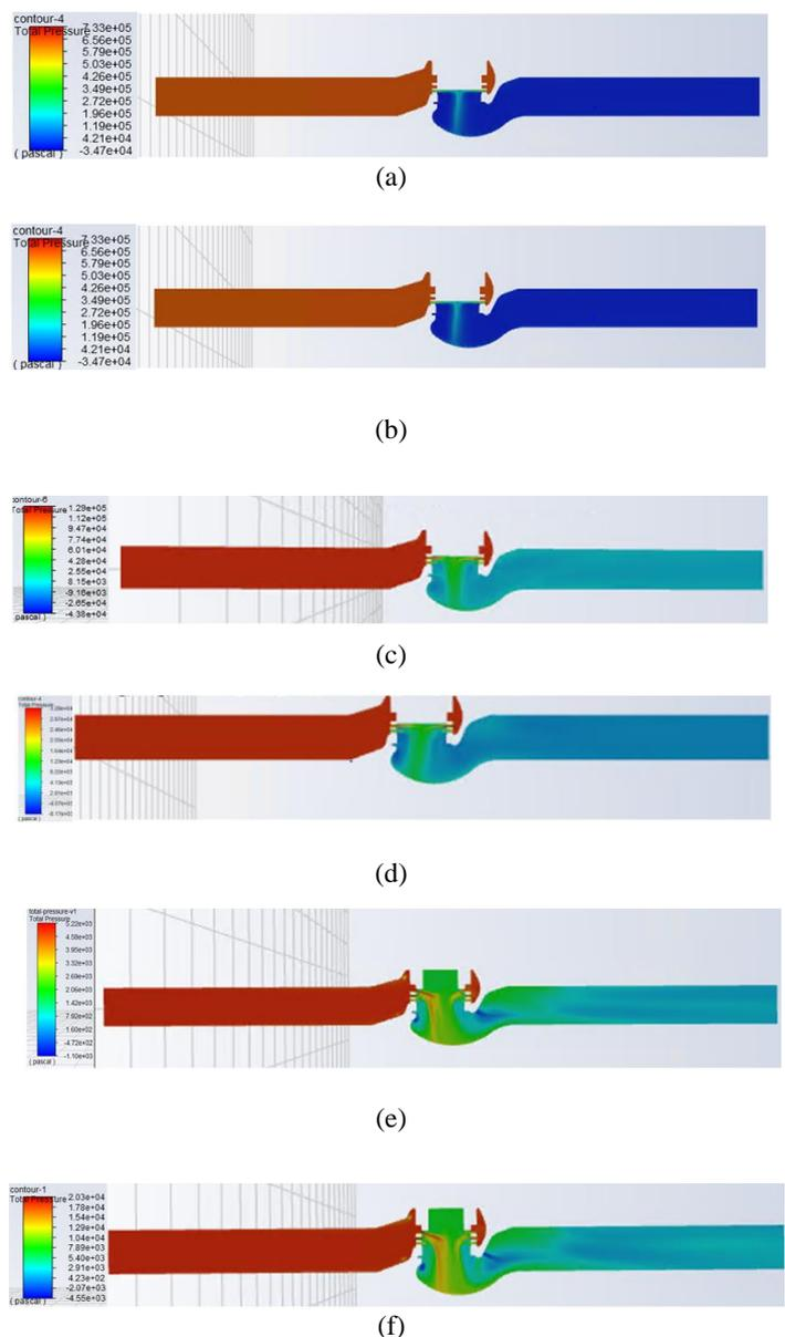
Figure 5: (a) (b) Contours of total pressure at 20% VOP with 1 m/s and 2 m/s velocity inlet, (c)(d) total pressure contours at 60% VOP with 1 m/s and 2 m/s, (e)(f) total pressure contours 100% open with 1 m/s and 2 m/s velocities at the inlet.
