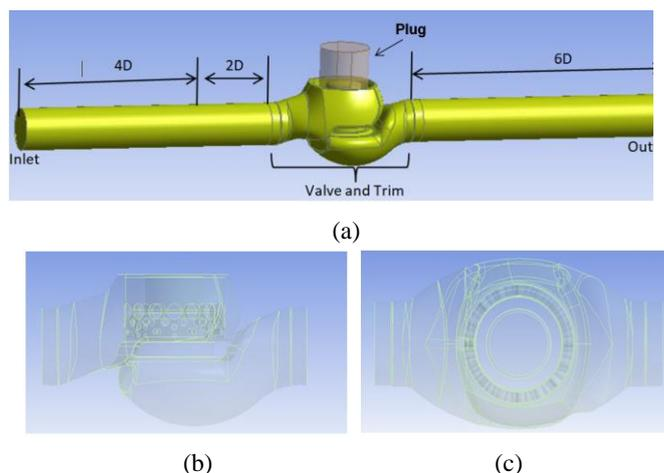
Figure 2: (a) Valve and pipeline flow domain geometry showing the pipe lengths according to the relevant BS standard (b) side view of the valve section (c) top view of the valve section
