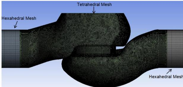
Figure 3: Mesh of the valve flow domain
