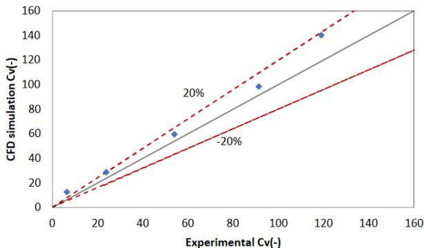
Figure 4. validation of numerical results of the valve's  $C_v$  with experiments.
