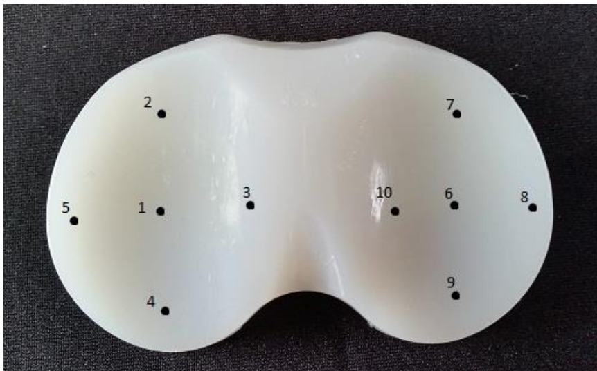
Figure 29 - Diagram showing the location of measurement points for surface topography study.
