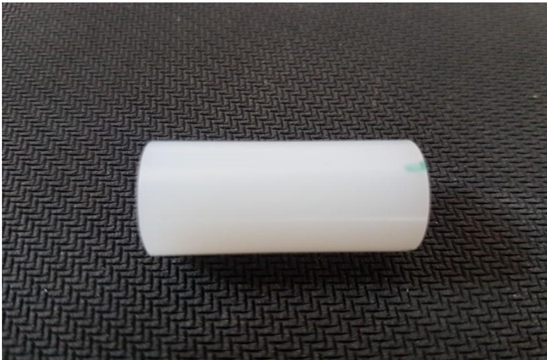
Figure 15 - Example of Scaling Artefact used in CT scans.
