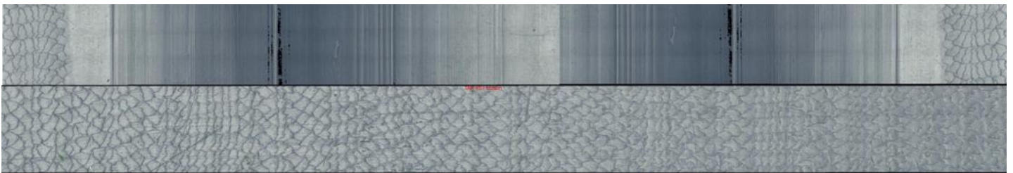
Figure 26 - Example of Surface Texture of Worn (TOP) and Unworn (BOTTOM) TAR components. Measurement taken using FVM.
