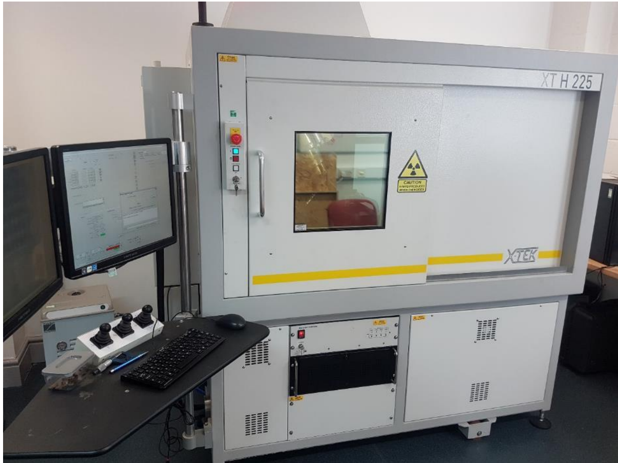
Figure 14 - NIKON XTH225 CT Scanner as used throughout this project.
