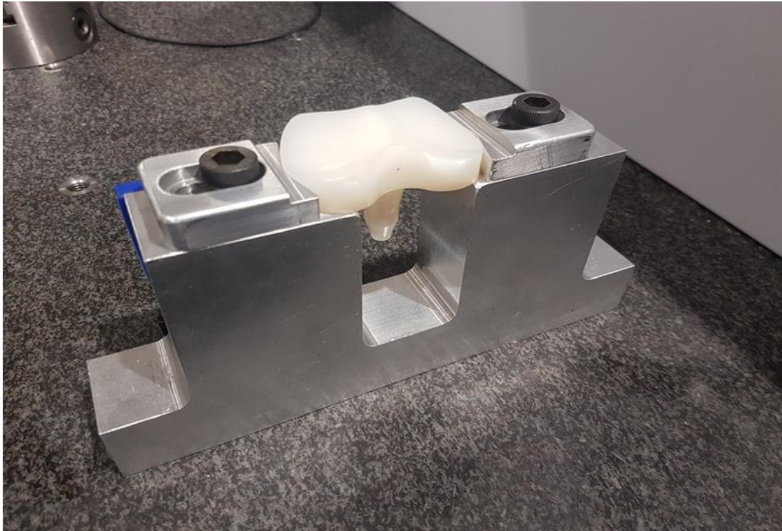
Figure 18 - Example of Fixturing used for TKR components on CMM.
