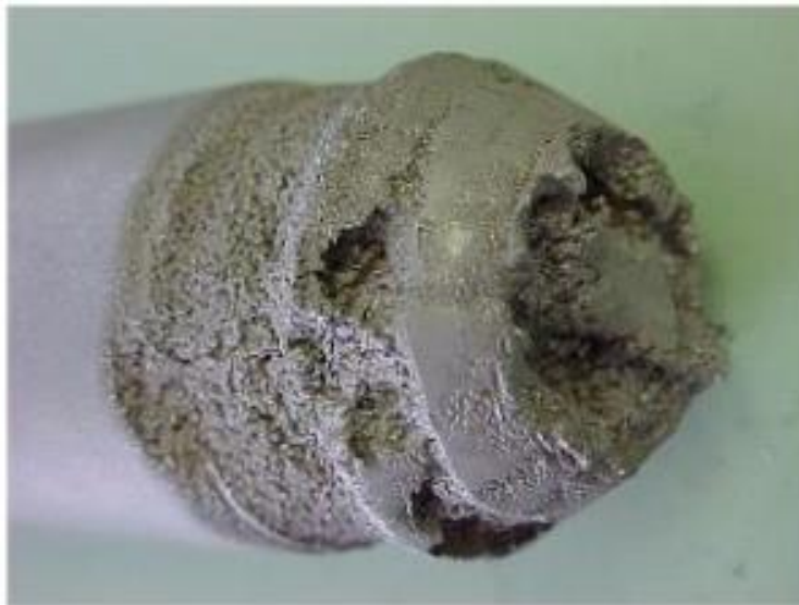
Figure 1-7: Extent of Cavitation Damage Within the Vicinity of a Valve Plug (Flotech, 904-358-1849, 2020) [103]
