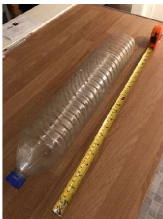
Figure 7.6 'In-house' sampling hood with extension piece
