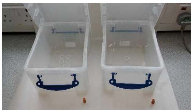
Figure 2.7 VOC sampling chambers chosen as optimum from the trials and preliminary experiments
