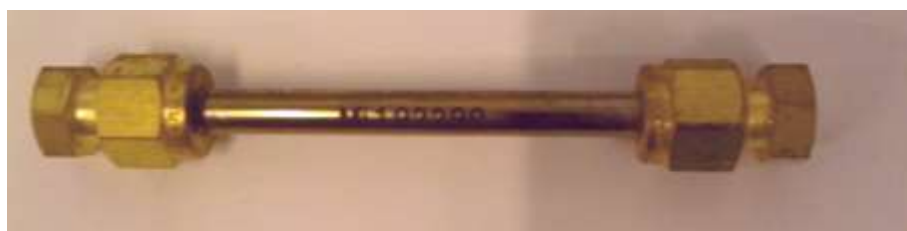
Figure 2.3 TD tube with brass storage ends attached
