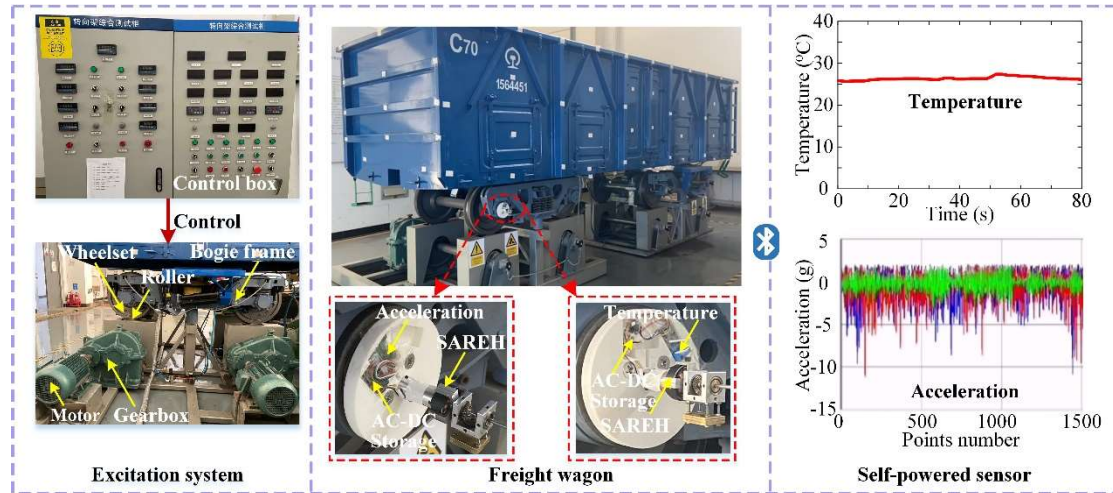
Fig. 14. Railway evaluation of the SAREH. Self-powered wireless shaft temperature and triaxial acceleration monitoring during the railway simulation tests.
