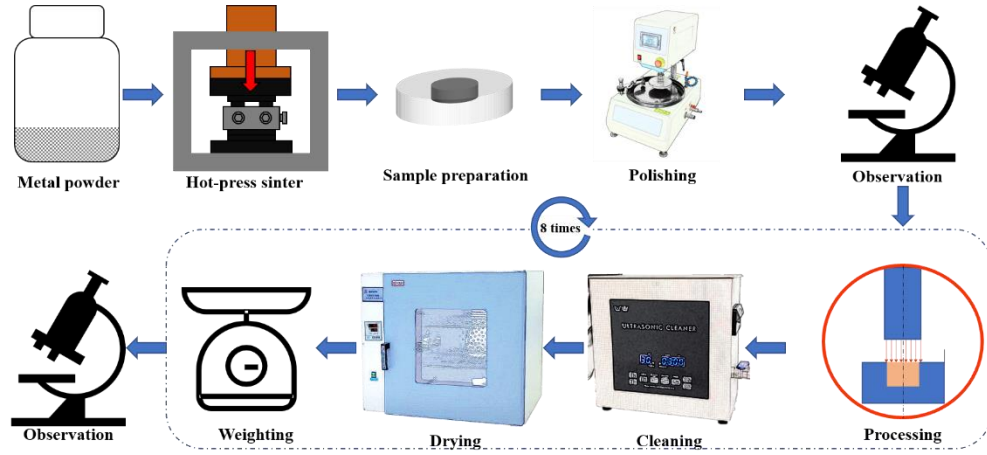
Fig. 2. Process schematic of jet biomachining experiment
