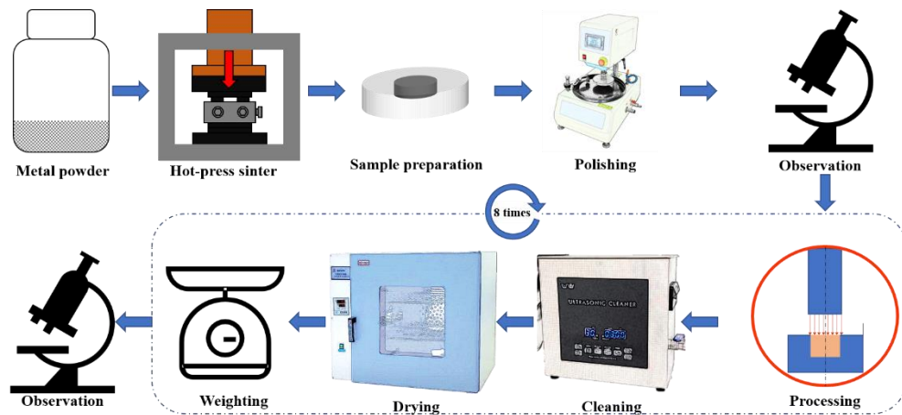
Fig. 2. Process schematic of jet biomachining experiment
