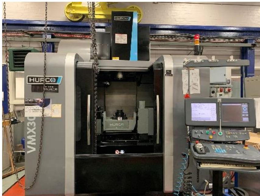
Figure 38. AC type 5-axis milling machine with moving bed
