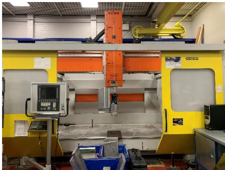
Figure 39. AC type of 5-axis milling machine with fixed bed
